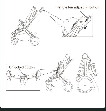
When the seat unit is used in the forward direction. To adjust the height of the handle, push the handle downward while pressing the handle adjustment button. Then, raise the footrest to the highest position.
