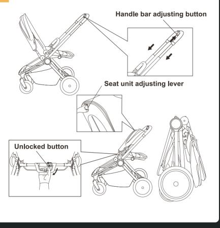
When the seat unit is used in the reverse direction. To adjust the height of the handle, push the handle downward while pressing the handle adjustment button. Then, adjusting the backrest level to the lowest position by moving it towards the front of the seat, closer to the handle bar.
