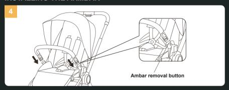
Inserting the armbar connecter inside the socket of the bar till the sound of "click". Indicating the correct installing way.
