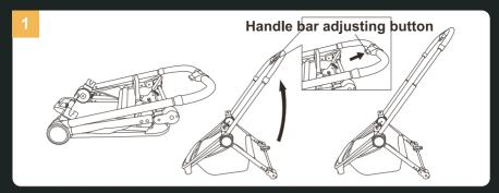
Lift the handle bar upwards until a "Click" sound, indicating the stroller is open completely.
