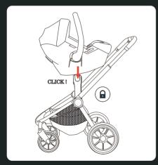
1b. To attach the baby carrier, place the baby carrier onto the adapters. Make sure the baby carrier is attached to the adapters properly.
