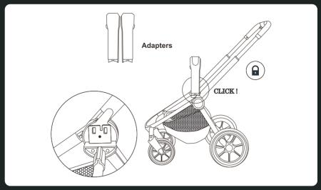
1a. Remove the seat unit from the frame to fit the adapters. To attach adapter, place the adapter onto mounts. Listen for a "click' sound indicating it is correctly assembled.
