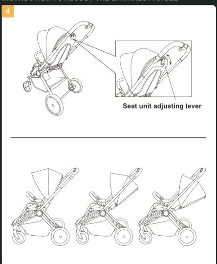
To recline the backrest, use the seat unit adjusting lever, and then adjust the backrest to a desired angle.
