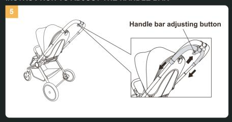
To adjust the height of the handle, pull the handle upward or downward while pressing the handle adjustment button
