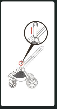
2b. To remove the adapter, by pressing the two release buttons. Remove the adapter as shown in the picture.
