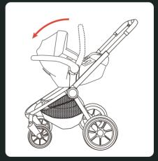
1c. Adjust the handle of the baby carrier by pressing the adjuster button at the side of the handle, moving down the handle as shown in the picture.
