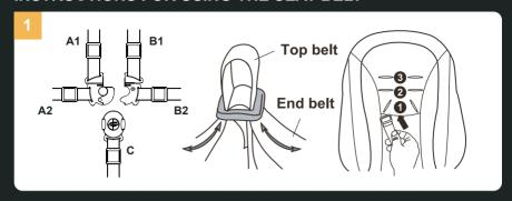
As shown in the picture, attach the A1 upper belt to the A2 lower belt, and attach the B1 upper belt to the B2 lower belt. Make sure that both Part A and Part B are locked, attach Part A and Part B together and attach to Part C.
